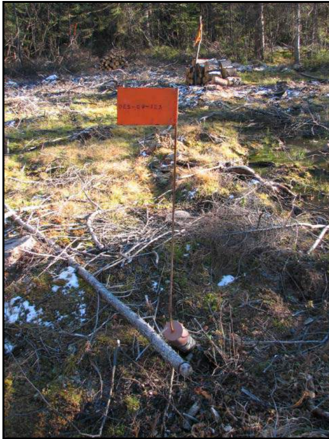
Figure 11.1 Diamond Drillhole Cap
